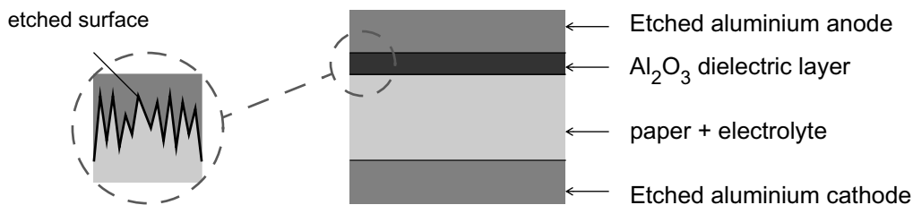
Figure 3.13 Electrolytic capacitor construction
